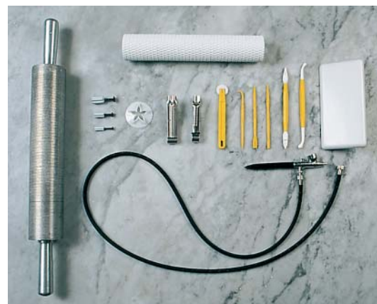
Marzipan tools. Top: basketweave roller. Middle row: metal rolling pin, small cutters with release plungers, strawberry leaf cutter, nippers, modeling tools, smoother for covering cakes with sheets of marzipan. Bottom: color sprayer.
